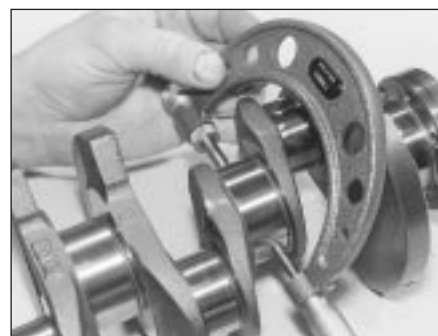
17.4 Measuring the main bearing journal diameters
