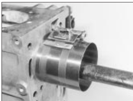
22.9 Refitting the piston and connecting rod assemblies, with the aid of a ring compressor
