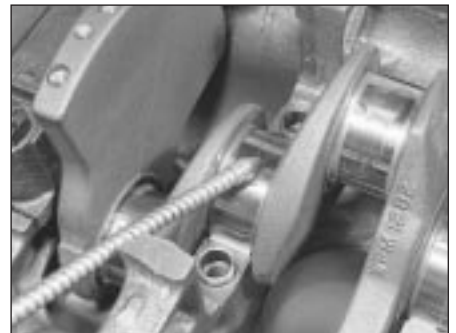
21.14 Thoroughly lubricate the crankshaft journals
