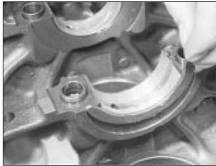
21.5 Fitting the crankshaft thrustwashers
