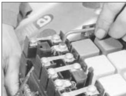
4.21b . . . undo the cable retaining screw . . .
