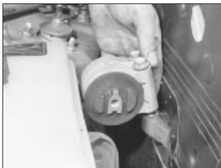
4.43 Remove the right-hand engine mounting
